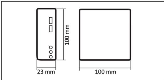
**KET-MUM-100.4G** is a device that integrates the latest generation of **4G-LTE modem**, a router and an **Ethernet output**.
