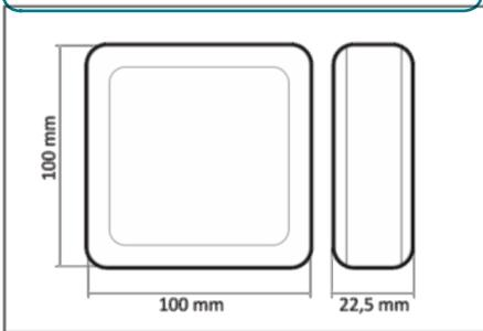
**KET-TLP-110** is an environmental sensor capable of detecting the movement of people within a radius of about 3-4 meters. The built-in **double light sensor** allows you to limit the lighting of lights only below a certain lighting threshold that can be set remotely. The temperature sensor completes the characteristics of the device.
